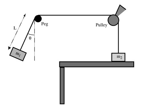
Figure 1: The two masses connected by a cord and pulley arrangement.
