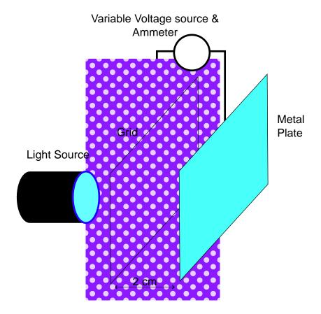
Figure 1: An apparatus to measure the photoelectric effect.
