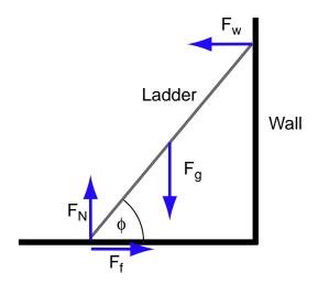
Figure 1: The forces acting on the ladder.
