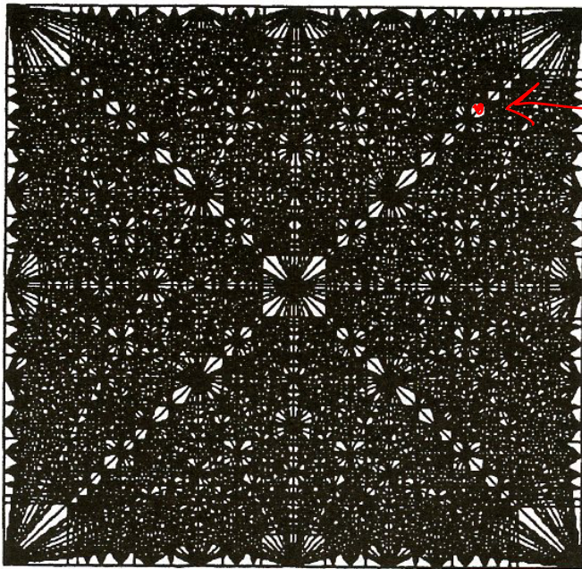
Figure 5.8. Resonance lines in the tune plane for ninth integer and below.
