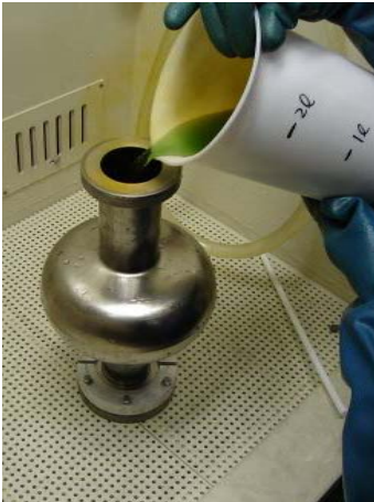
Figure 5: Light Chemical Polishing.
