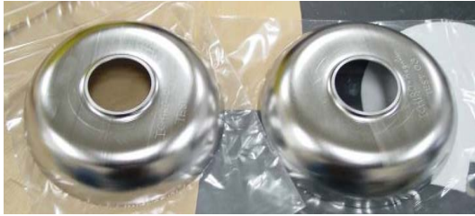
Figure 2: Trimmed, deep drawn, pure niobium half cups.
