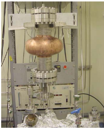
Figure 9: Cavity assembled ready for cold testing.
