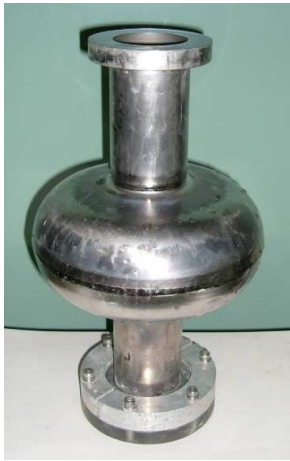
Figure 3: Assembled single cell cavity structure.
