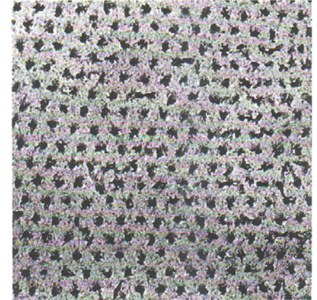
Figure 19 Triangular lattice of fluxoids through top surface of a superconducting cylinder. The points of exit of the flux lines are decorated with fine ferromagnetic particles. The electron microscope image is at a magnification of 8300, by U. Essmann and H. Trüble.
