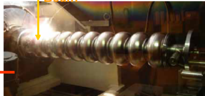
EBW of end-beam-pipes and cell-part
