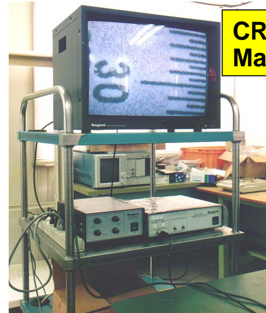
KEK Inner surface inspection system
