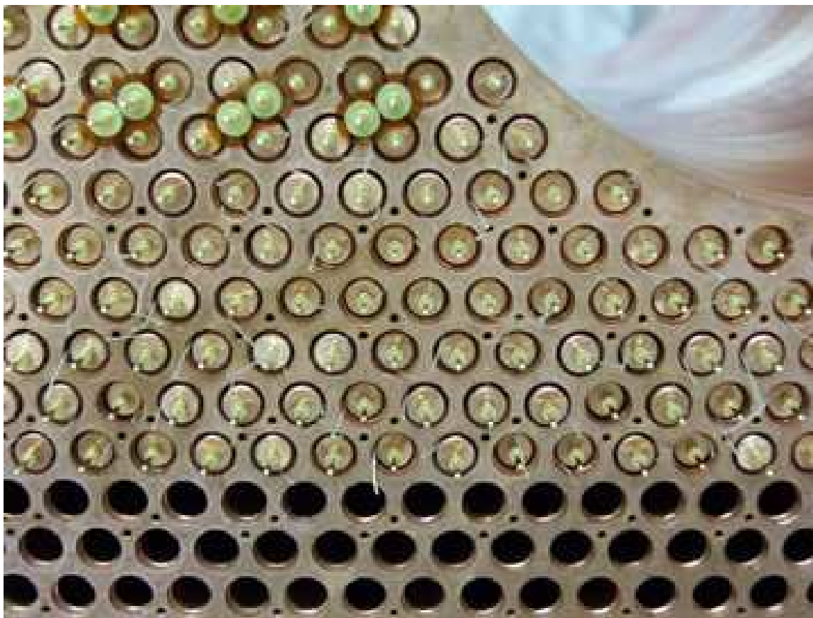
Figure 5. Photo of the front face of the FCal1 module during construction. The beam hole is partially visible in the upper right.
