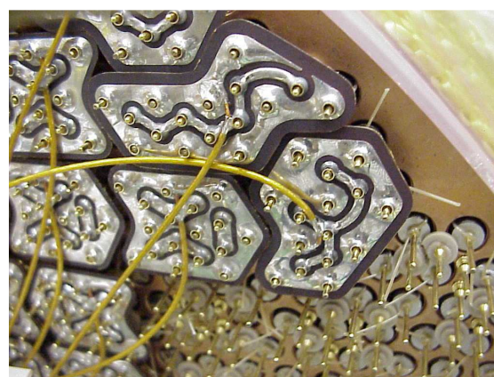
Figure 18. Photo showing both regular and irregular interconnect boards mounted on signal and ground pins of FCal3.
