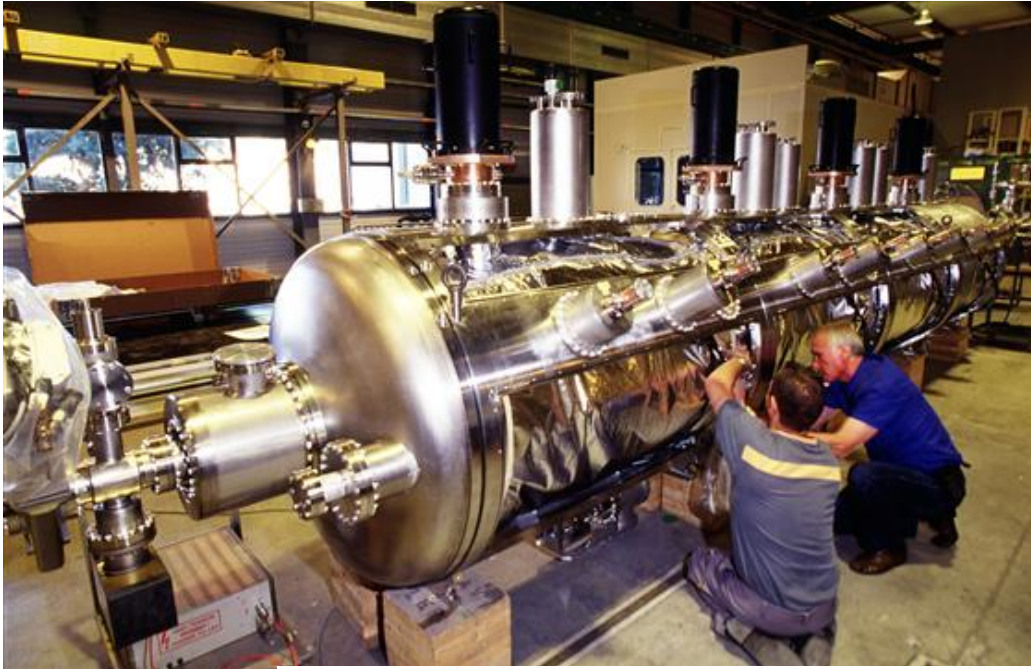
A voltage generator induces an electric field inside the RF cavity. Its voltage oscillates with a radio frequency of 400 MHz.
