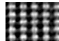
Atoms of silicon spacing 0.078 nm
