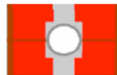
2-layer winding without spacers in body or ends
