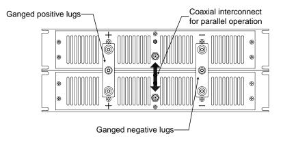
In addition to the ganged lugs, the coaxial connectors on the rear of each Model 601 must also be connected. If more than two units are connected in parallel, the middle units may be connected to the coaxial cable by using standard BNC "T" adaptors. The "end" units should be connected directly to the coaxial cable — no BNC "terminators" should be used.
