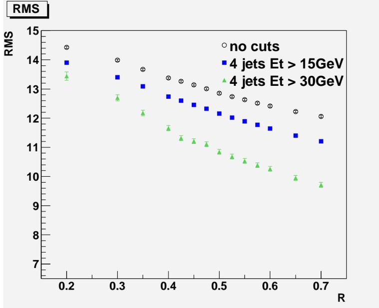
Figure 6: The RMS width of the invariant mass distribution for the dijet system as a function of cone size.
