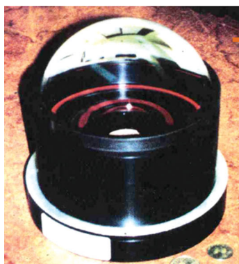
FIG. 32 (color). The F/1 wide-field CCD camera being mounted at the Anglo-Australian telescope.
