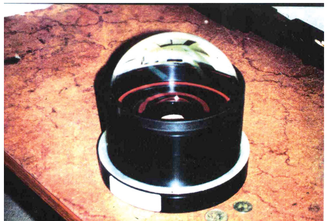
FIG. 7 (color). The novel F/1 wide-field CCD camera we developed for the Anglo-Australian 4-m telescope (AAT) to collect a wide enough field to search for z > 0.3 type Ia supernovae in hundreds of galaxies with each image.
